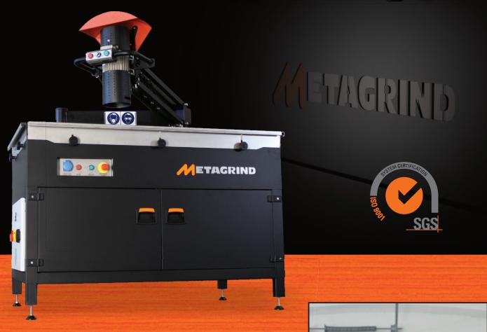
Manually operated machine designed for — deburring removing and dulling edges of sheet and metal parts after cutting, laser fusions, burned with plasma and flame. The working tool is a rotating head with two positions, equipped with a deburring grinding disc on one side on the other side with lammels deburring brush.
